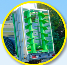
Large-diameter vertical beaters with retractable blades and HARDOX 450 teeth
